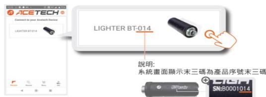
D. Instruction for binding: when the cell phone connects Lighter BT for the first time, pairing binding of the device must be executed first.
